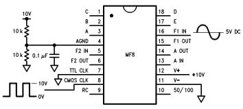
(a) MF8 Driven with CMOS Logic Level Clock
