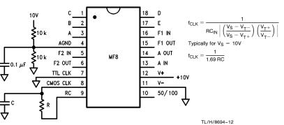
(c) MF8 Driven with the Schmitt Trigger Oscillator
