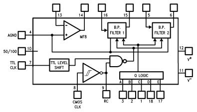
FIGURE 1. Simplified Block Diagram of the MF8
