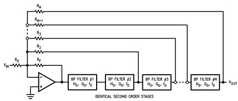
FIGURE 6. By adding more second-order filter stages and feedback resistors, higher order multiple-feedback filters may be built.
