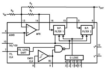
FIGURE 2c. Multiple Feedback Loop Connection
