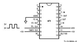
(b) MF8 Driven with TTL Logic Level Clock
