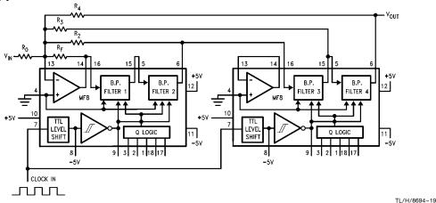
FIGURE 11. Eighth-Order multiple-feedback bandpass filter using two MF8s. The circuit shown accepts a TTL-level clock signal and has a clock-to-center-frequency ratio of 100:1.
