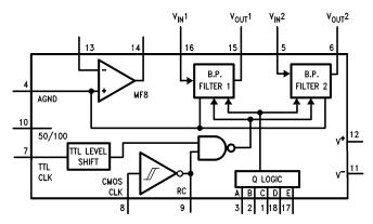
FIGURE 2a. Separate Second-Order "Tracking" Filters
