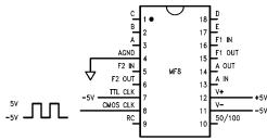
$_{\rm TL/H/8694-7}$  (a) MF8 Driven with CMOS Logic Level Clock
