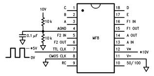
(b) MF8 Driven with TTL Logic Clock
