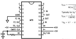
(c) MF8 Driven with Schmitt Trigger Oscillator FIGURE 3. Dual Supply Operation
